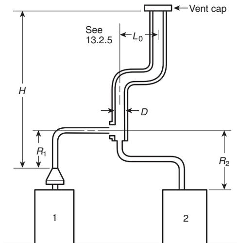
Asbestos cement Type B or single-wall metal pipe vent serving two or more draft hood-equipped appliances. [See Table 13.2(e).]
