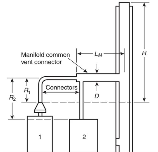
Example: Manifolded common vent connector  $L_M$  can be no greater than 18 times the common vent connector manifold inside diameter; that is, a 4 in. (100 mm) inside diameter common vent connector manifold should not exceed 72 in. (1800 mm) in length. (See 13.2.4.)
