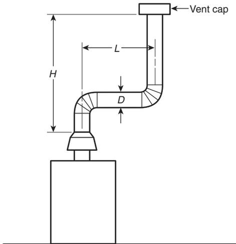
Asbestos cement Type B or single-wall metal vent serving a single draft hood-equipped appliance.
