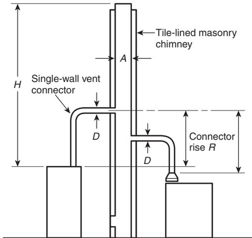
Table 13.2(d) is used when sizing single-wall metal vent connectors attached to a tile-lined masonry chimney.
